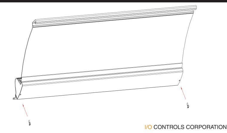
Step 9 - Install the screws back to the panel.
